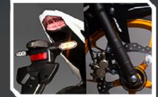
NEW ANTI-LOCK BRAKING SYSTEM (ABS) + NEW EMERGENCY STOP SIGNAL (ESS) The new ABS feature provides a more stable braking system to prevent wheels from locking during sudden brake or slippery road conditions; while the new ESS feature automatically blinks the hazard light to give early warning to drivers behind when sudden stop occurs.
